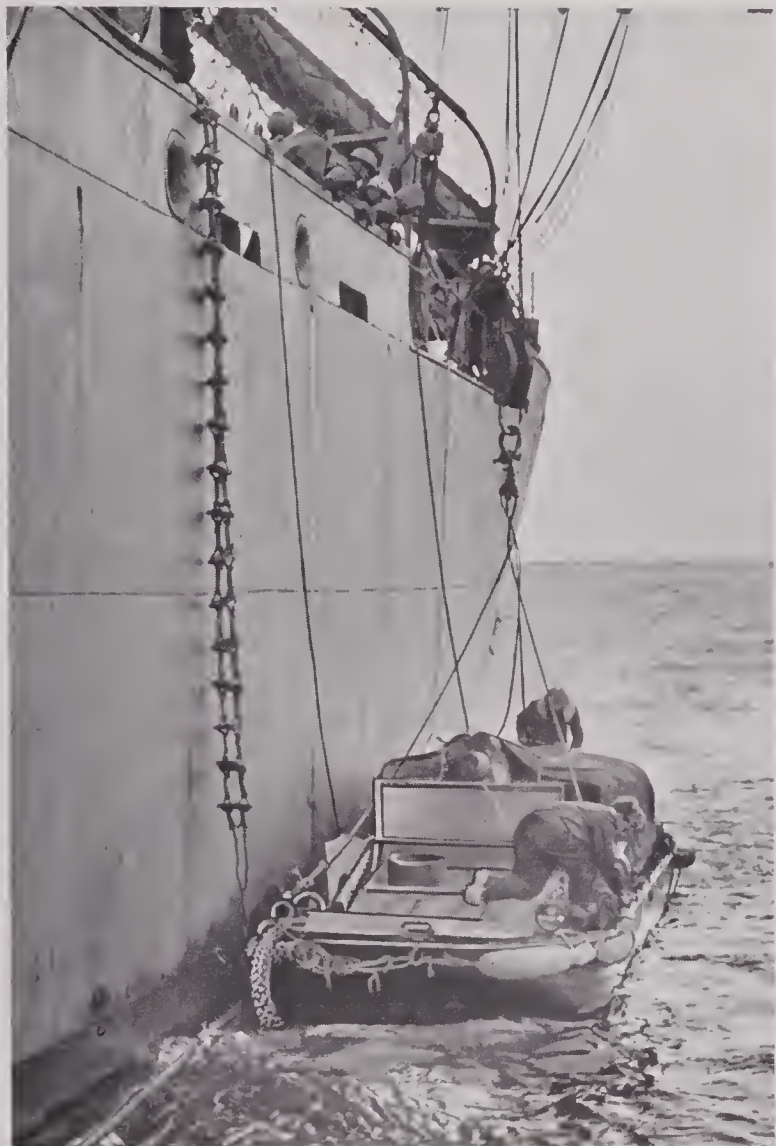
FIGURE 103. DUKW alongside Liberty ship with DUKW lifting sling being made fast.
